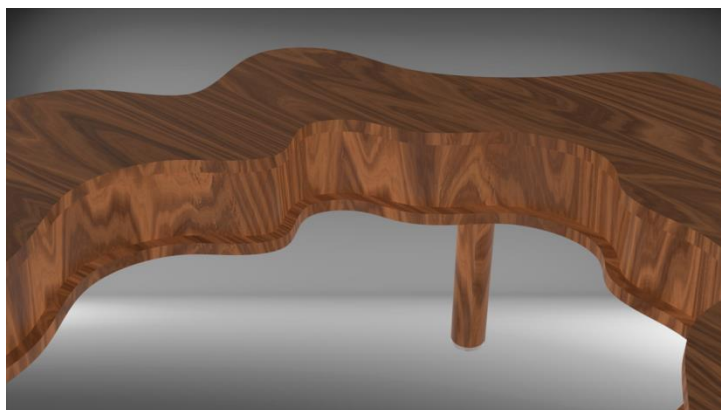
Fig. 75 - Pormenor do local para colocar as fitas LED
