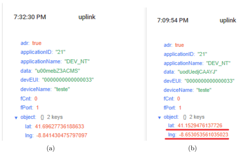
Figure 5.4: Device UPLINK to LoRa Server before and after GPS Spoofing. a) Real coordinates; b) Spoofed coordinates.
