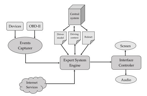
Figure 3. Architecture of the ADAS prototype.
