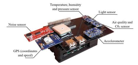
Figure 4. Raspberry-Pi connected to the PCB containing all the sensors.
