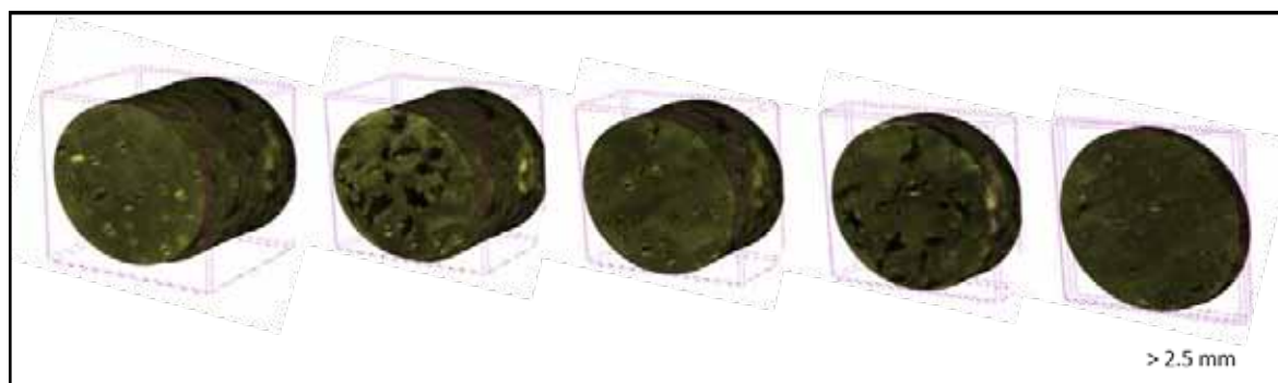
Fig 5. 3 – D reconstruction using CTvox version 3.0.0r1114 (64-bit). Image on the left represents a complete sample and image on the right represents a volume of interest (VOI).
