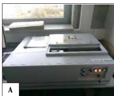
Fig. 2. A – QTRS-01X Data Analyser and Scanner (Quintek Measurement Systems Inc., Knoxville, TN, USA); B – Cassette where the sample is positioned.
