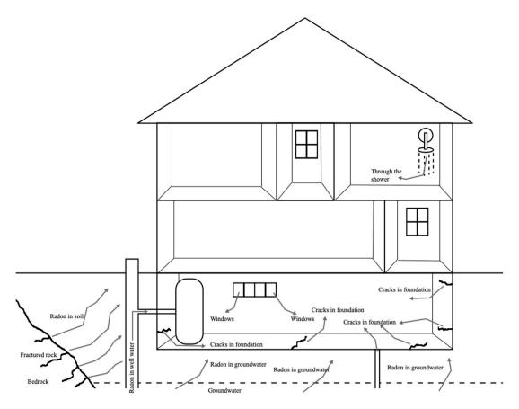
**Figure 3.** Radon can enter into buildings through cracks in the building structure after being released from rocks to soils and water. Water can transport radon into the buildings, as being highly soluble in cold water, this solubility is highly reduced in hotter water, being immediately released, for example, during showering (adapted from [43–46]).
