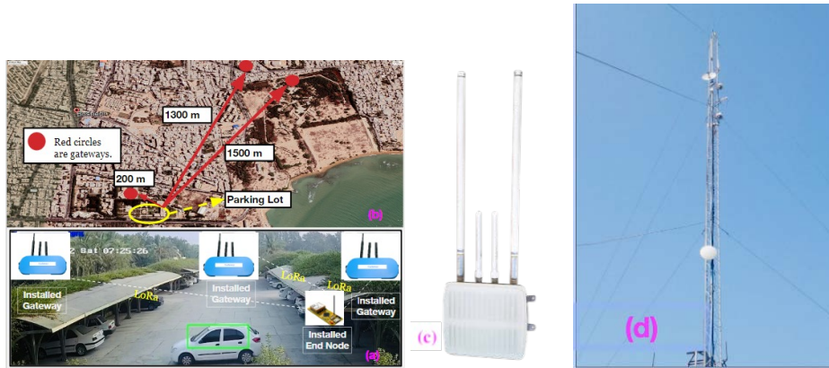
Figure 3: Experimental Setup. From left to right: (a) Experimental setup in a parking lot where measurements were collected from 16 different end node positions. (b) The bird’s eye view (taken by Google Maps) of the entire area identifies the location of the gateways, their precise distances where they are installed, and the location of the parking lot. (c) LoRaWAN gateway that is assembled with Lora Radio and LoRaWAN Antennas (d) An example of a tower where LoRaWAN gateways are installed (In total, three gateways are installed on three towers shown in (d)).
