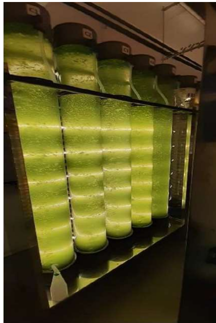
Figure 14.9. Airlift type vertical column photobioreactor
