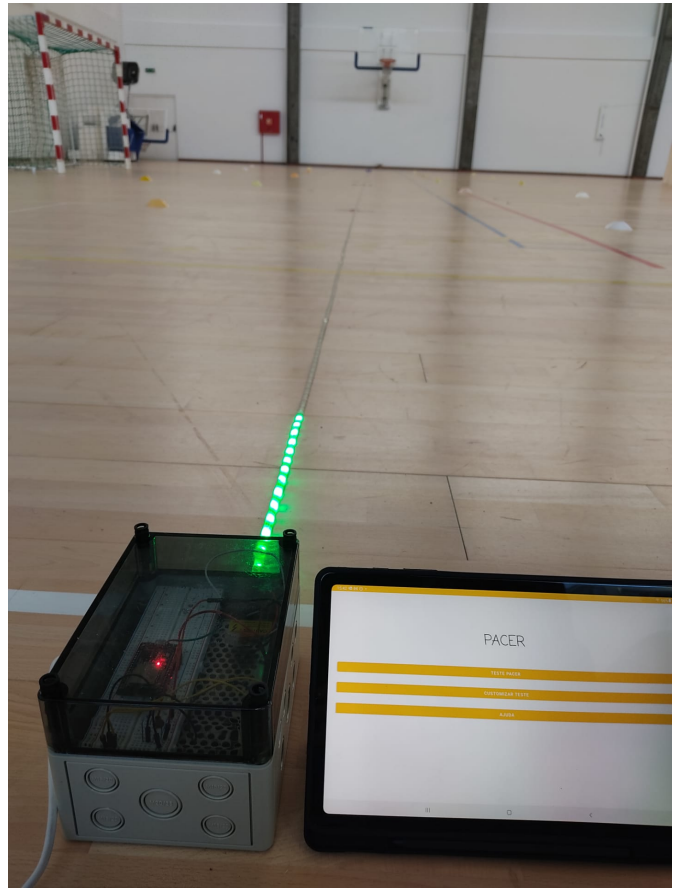
Fig. 4. Prototype on operation. The controller is ready and waiting for an instruction from the Android device.
