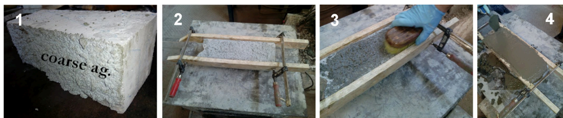
Figure 3. Some phases of the coating process: coarse aggregate and four faces sealed with paraffin (1); preparation of the formworks (2); coarse aggregate moistening (3); application of the first base coat (4).
