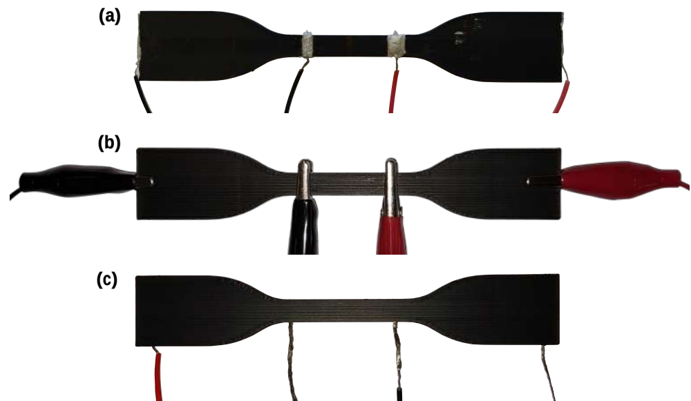
Figure 3. Normalized tensile testing specimen with different variants of electrical connections (bonding): (a) Silver paste and silver paint; (b) crocodile clips; (c) inlaid during printing.
