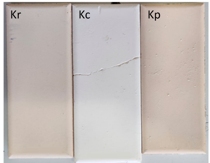
Fig. 5. Samples photographs fired at 1190 °C, for the visual coloration analysis.
