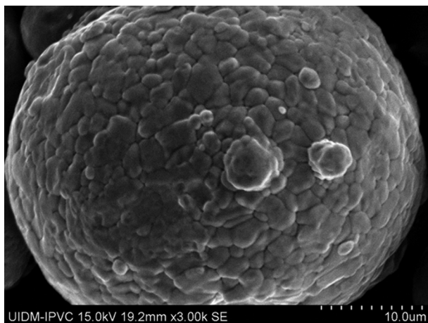
Figure 5. Scanning electron microscopy image at 3000× magnification of Tool Steel 1.2709-A LMF (TRUMPF) powder particle Abbreviation: SEM: Scanning electron microscopy
