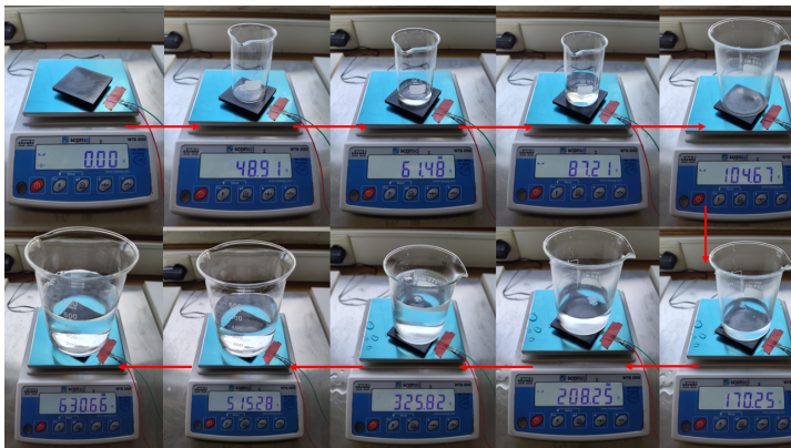
Figure 11. Representative sequence of the FSR calibration process using incremental water loading. The beaker mass was progressively increased while the corresponding ADC values were recorded with the ESP32.
