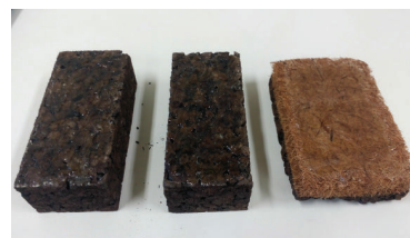
Figure 2: black cork (high and low densities) and coconut fiber trials with pine rosin applied superficially.
