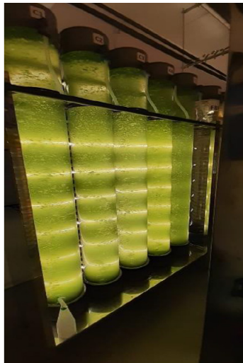
Figure 14.9. Airlift type vertical column photobioreactor
