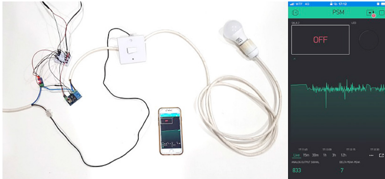
Figure 10.12. Result: lighting off
