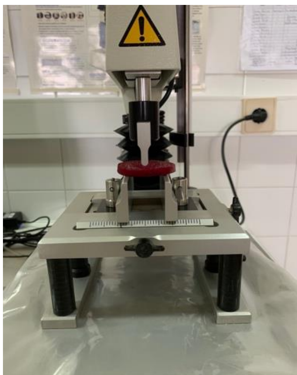
Figura 12. Ensaio com a sonda Three Point Bend Rigs HDP/3PB (Forward Extrusion cell) com amostra de beterraba.
