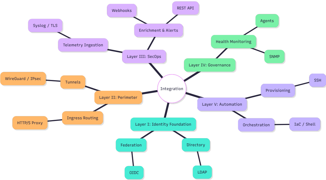
Figure 5.3: Framework integration and protocols map, illustrating the open standard communication protocols (e.g., OIDC, LDAP, REST API, SSH) employed between architectural layers to prevent vendor lock-in.
